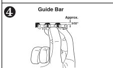
Pull chain to check tension. Guide links should not come out of guide bar groove...
